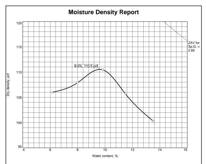
Test specification: ASTM D 698-Method B Standard
