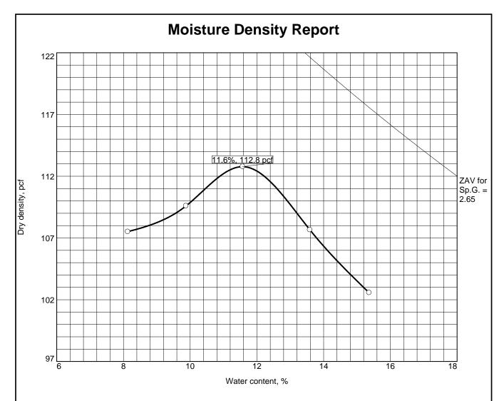
Test specification: ASTM D 698-Method B Standard
